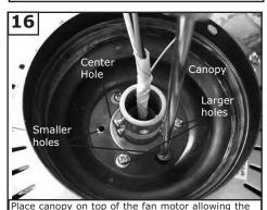
yoke to pass through the large hole in the center of the canopy. Align the 3 larger holes around the center hole with the 3 screws already installed in the fan. Install 3 flush mount screws provided into smaller holes and tighten securely.
